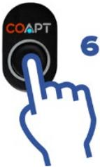
**Double beep after the button has been held for 6 seconds (LED is solid CYAN for the first 2 seconds and flashing CYAN from 2 to 6 seconds.**
