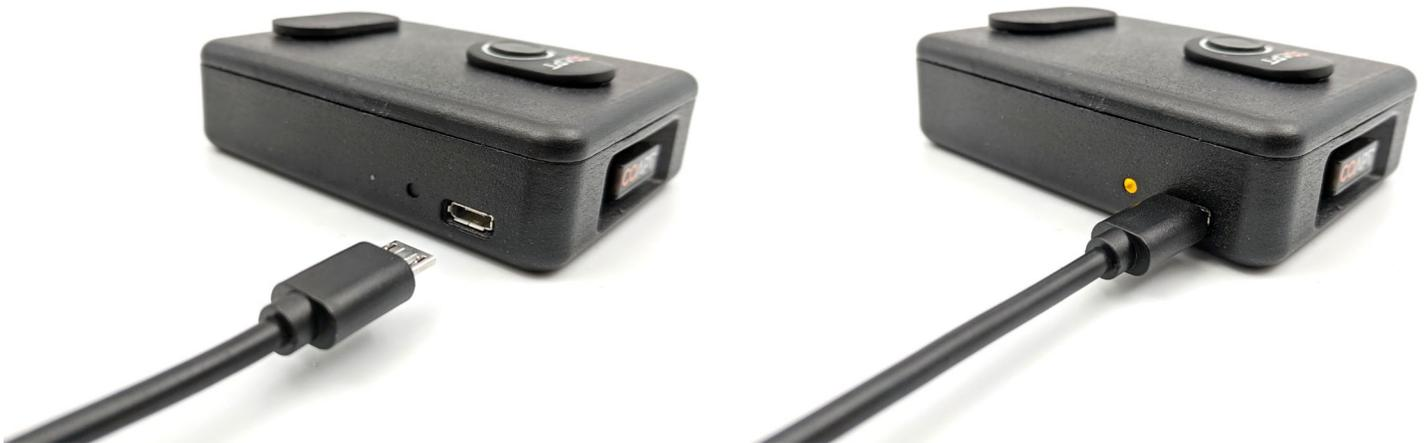
The Charging Status Indicator LED Light is next to the Evaluation Kit’s micro-USB port has three different colors:
